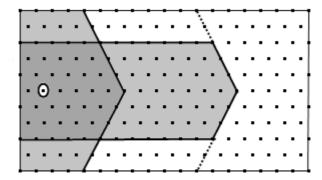
**Figure 6**: When the size of the structuring element is higher than half the size of the window (here, size is 12 whereas window height is 11), edge effects are unavoidable.
