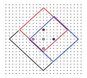
Figure 10: Boundary overlapping: the boundaries of the size 7 diamonds generated by the red and blue pixels overlap, which insures that no boundary point of the final size 10 diamond is missing.
