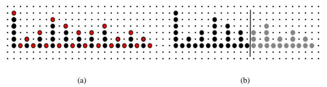
**Figure 1**: (a) successive dilations of an initial point (top line) by doublets of points of respective sizes 6, 8, 4, 2 and 1. In red, points added at each step. (b) Verification that no edge effect may occur.
