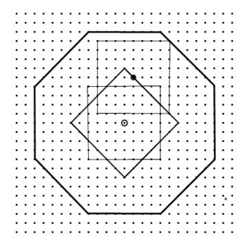
**Figure 11**: Size 10 octogon obtained by a size 6 sparse conjugate square dilation followed by a size 4 square dilation. We see that the dilations of the center point and of the boundaries of the conjugate square are sufficient to get an octogon without holes.
