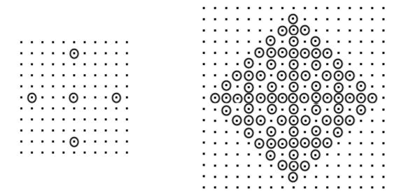
**Figure 8**: "Cross" structuring element of size 4 (left) and result of successive dilations of a point by this structuring element (sizes 4, 2 and 1) producing a sparse conjugate square of size 7 (right).
