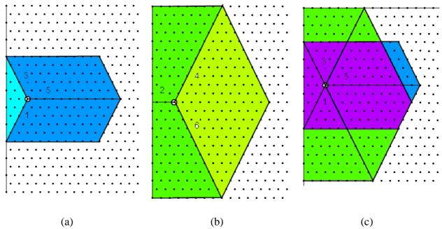
**Figure 3**: (a) Dilation of a point near the edge by three successive dilations by segments in directions 1, 3 and 5. (b) Same operation with segments in successive directions 4, 6 and 2. (c) The union of these two results do not prevent edge effects when the initial point is in the upper left corner.
