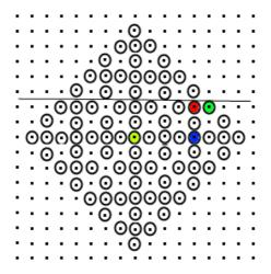
**Figure 9**: The green pixel on the diamond boundary at coordinates (5, 2) is generated by a size 1 dilation of the red pixel, itself obtained by a size 2 dilation of the blue one. The blue pixel has been generated by a size 4 dilation of the initial yellow center point. These points are always propagated inside the image window (refer to the possible position of an edge indicated by an horizontal line in the figure).
