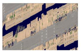
Figure 4: Lidar point cloud viewed in sensor-space: horizontal axis corresponds to time and vertical axis corresponds to rotation angle.
